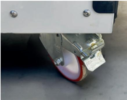
**RUOTE PIROETTANTI, LE POSTERIORI CON SISTEMA FRENANTE, PER LA MASSIMA MANOVRABILITÀ**
